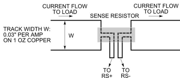
**Figure 1:** Making PCB Connections to the Sense Resistor.
